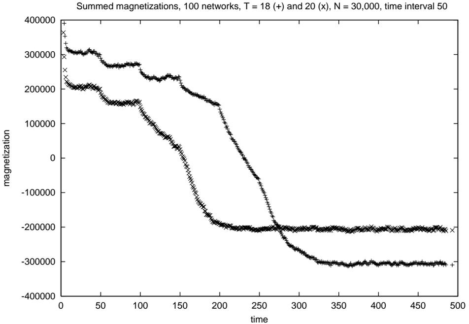
Fig. 3. Total magnetization versus time, summed over 100 networks of  $N = 30,000$  when after every 50 iterations the most-connected free spin is forced down permanently. For lower temperatures, the sign change of the magnetization happens later.  $N = 2,000,000$  gives similar effects.
