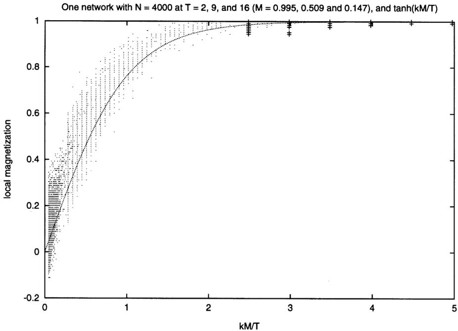
Fig. 2. Correlation between the number of neighbours and the local magnetization  $\langle S_i \rangle$  for one network of  $N=4000$  at  $T=2, 9$  and  $16$  ( $M=0.995, 0.509$  and  $0.147$ ), and  $\tanh(kM/T)$ . Average over  $250 < t \leq 500$  iterations. The curve is the mean field prediction  $\tanh(\beta kM)$ .  $N=2,000,000$  gives similar effects.
