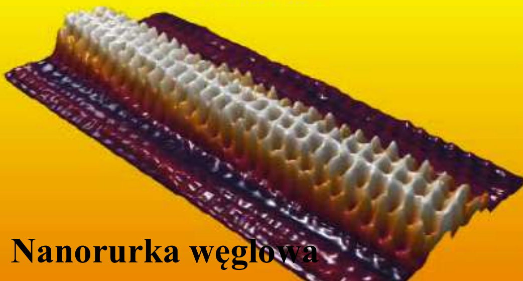
STM image of a Single-Wall Carbon Nanotube
