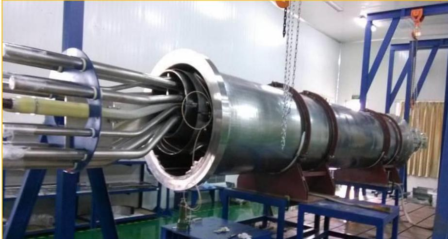
Internal components of a cryostat feeder prototype.
