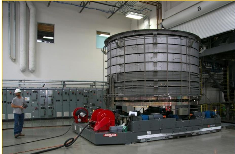
Module tooling stations are in place and being commissioned, including the heat treatment furnace shown here.
