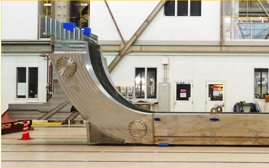
Connection of segments for the first inboard Toroidal Field Coil structure (completed in November 2015), a significant achievement for TF coil procurement.
