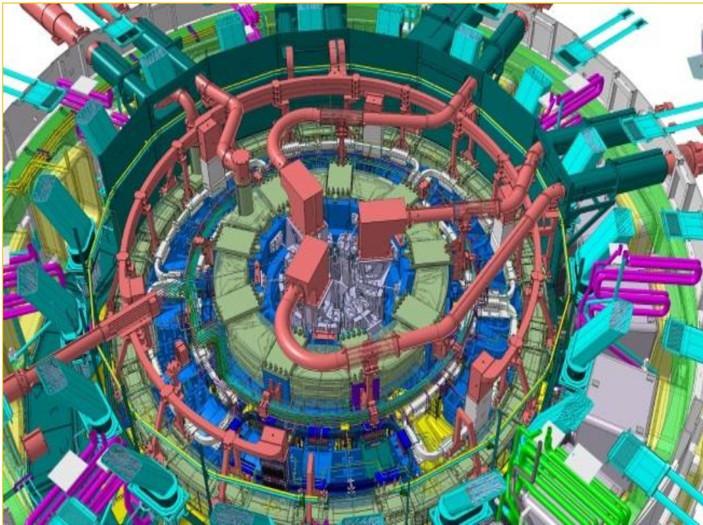
A top view of the cryostat illustrates the high density of sensitive equipment to be installed (e.g., magnet feeders shown in brown, blanket water pipes shown in light blue). A clash free design as well as the access to install and if needed maintain the systems must be ensured by the integration team.
