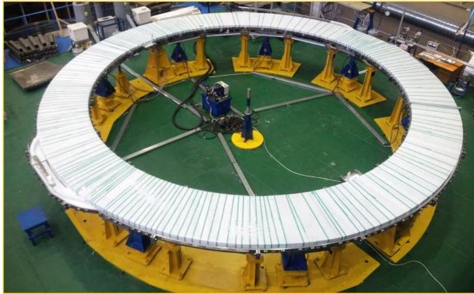
Fabrication and qualification tests of PF1 winding pack stack sample were successfully completed.
