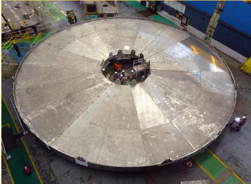
India is responsible for fabrication and assembly of the 30x30 meter ITER cryostat. The base plates were delivered to ITER in December 2015.
