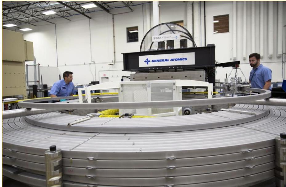
General Atomics is fabricating the 1000-ton Central Solenoid (CS). In April 2016, winding of the first CS module was completed.
