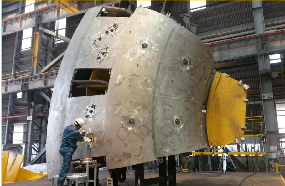
At Hyundai Heavy Industries, where 2 of 9 vacuum vessel sectors are under construction, welding on the upper section of the inner shell for Sector #6.
