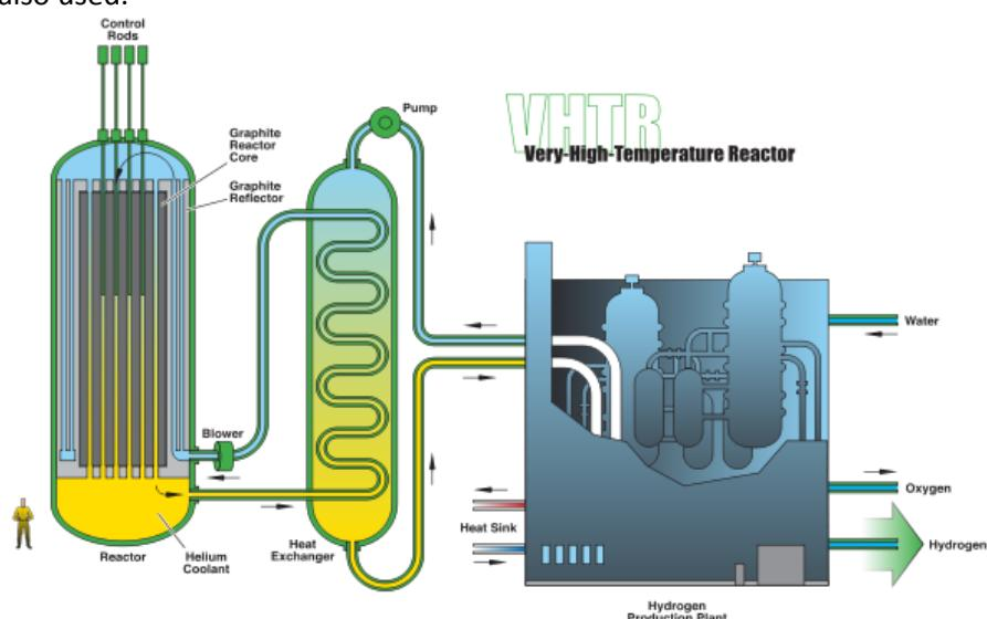
Fig. 5. Scheme of HTR reactor. [1]
