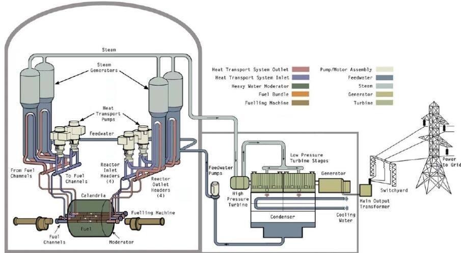
Fig. 3. Scheme of CANDU reactor. [2]
