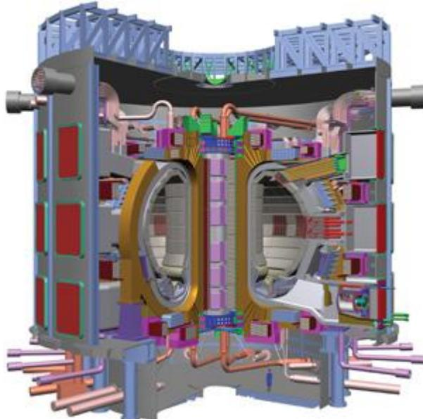
*Fig. 6. Scheme of ITER vacuum vessel. [3]*
