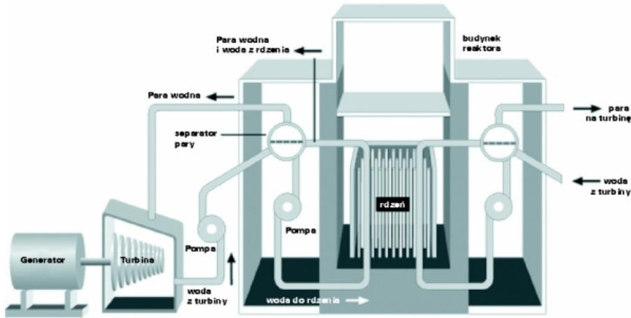
Fig. 4. Scheme of RBMK reactor. [2]
