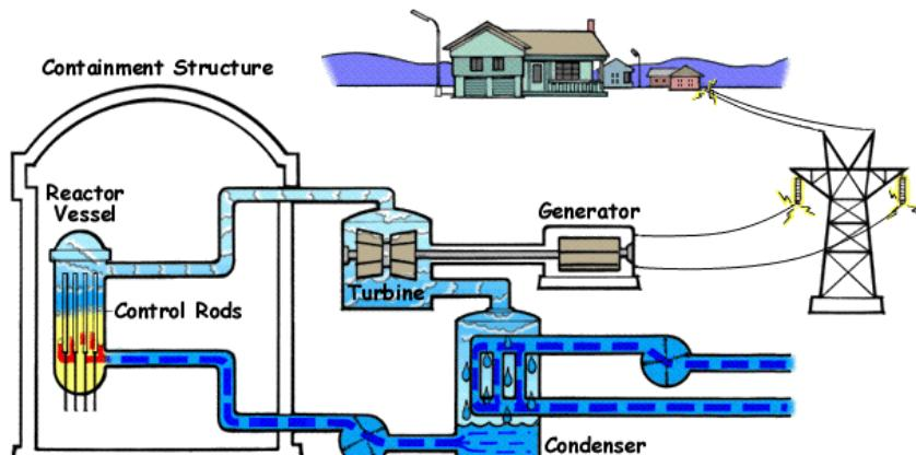
Fig.2. Scheme of BWR reactor. [1]
