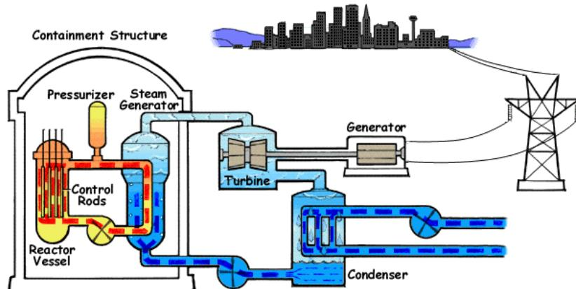
Fig1. Scheme of PWR reactor. [1]
