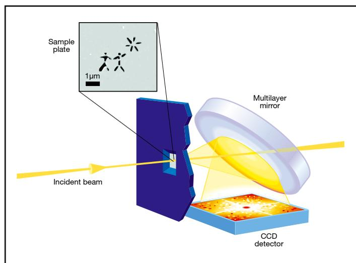
Schematic representation of the flash diffractive imaging experiment at the FLASH free-electron laser
