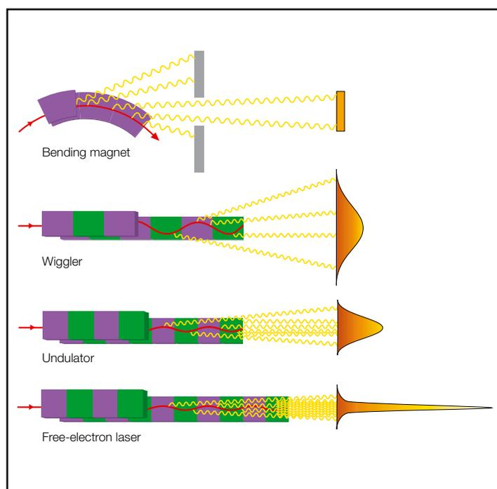
Generation of radiation in various types of magnet structures
