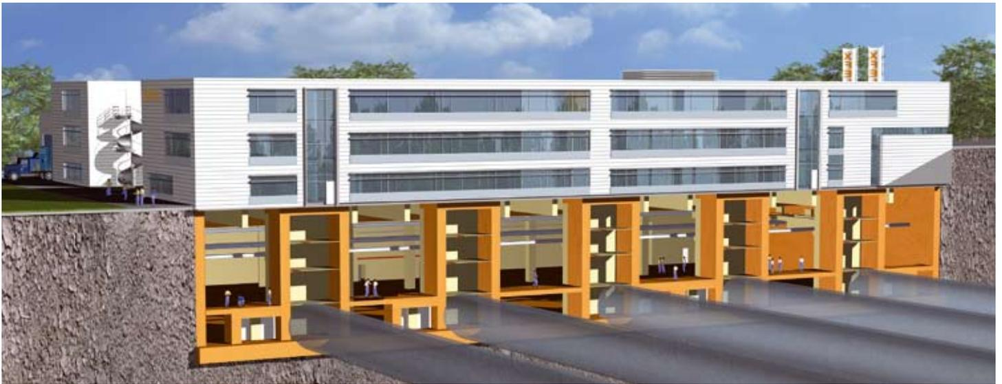
The main building on the XFEL research campus with the underground experimental hall in the planning stage: The photon tunnels, from which the laser-like X-ray flashes of the XFEL are led to the experimental stations, terminate in this subterranean hall.
