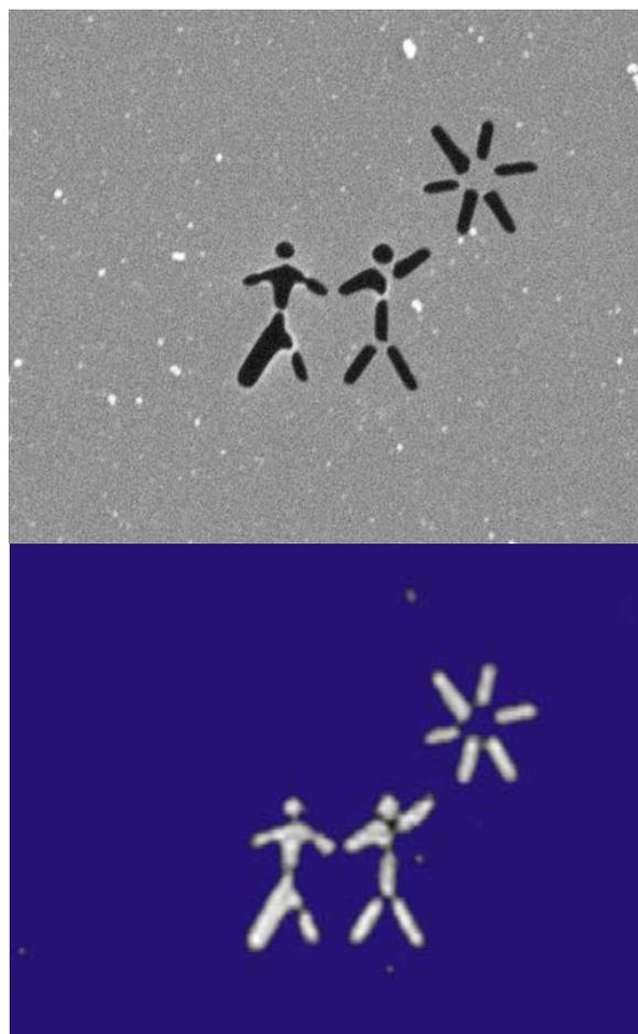
Top: The sample under the scanning electron microscope – two stick figures under a sun, cut into a membrane with a thickness of just a few nanometres
