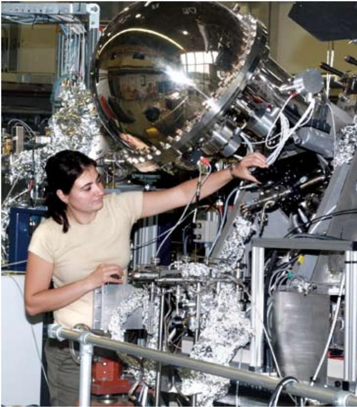
● In the HIXSS experiment, the intense laser light from FLASH is used to explore catalytic processes on solid-state surfaces.
