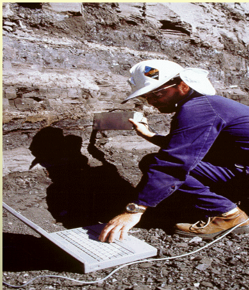
Low activity portable coal face ash analyser for differentiating coal and look alike sediments. The use of quantitative face ash analyser permits selective mining and is applicable to the production phase in open-cut pits and underground mines. The analyser works as a backscatter gamma ray type gauge.
