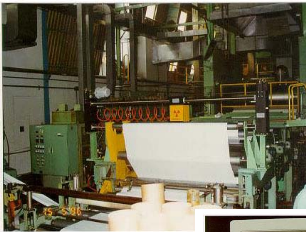
GLASS SHEET THICKNESS GAUGE ( Am-241 Gamma backscattering)
