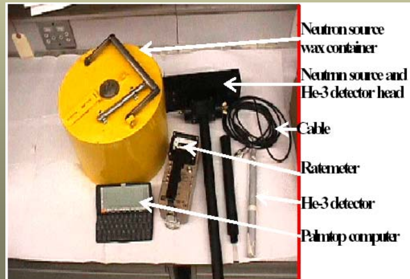
Typical neutron backscatter gauge equipment
