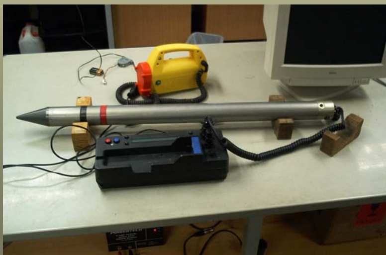
Low activity portable coal face ash analyser for differentiating coal and look alike sediments. The use of quantitative face ash analyser permits selective mining and is applicable to the production phase in open-cut pits and underground mines. The analyser works as a backscatter gamma ray type gauge.
