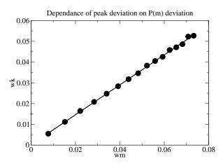
Fig. 6. The relation between the peak width wk (a standard deviation of peaks in  $P(\ln k)$ ) and the distribution width wm (a standard deviations of  $P(\ln m)$ ). The slope of the line is  $\alpha = 0.722$ .
