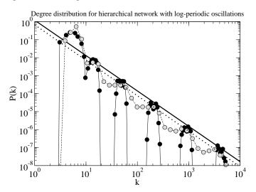
Fig. 2. Degree distribution for two networks with different  $P_{\rm M}(m)$ . Filled circles are for m = 3 or 4 with equal probability, gray circles are for uniform m distribution between 1 and 5. The straight lines show scaling of peak heights and correspond to  $\gamma = 0.967$  for the first case (continuous line) and  $\gamma = 0.973$  for the second (dotted line).
