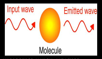
and then emits its own light wave that interferes with the original light wave.
