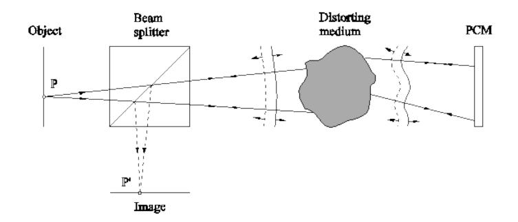
Basic two-pass geometry for imaging and aberration correction using a PCM(Phase conjugate mirror).
