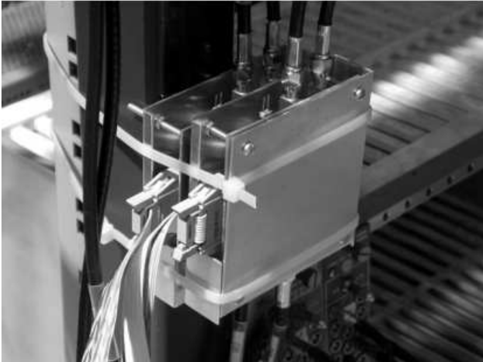
Figure 1.43: Photograph of the shoebox prototype (for two input channels) tested at CERN PS in June 2004. The input cables are seen entering from below and the output cables exit from the top. The ribbon cables deliver \pm 6 V of power.
