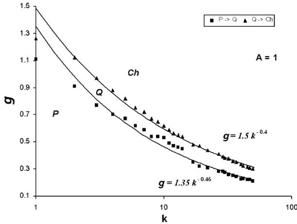
Fig. 8. The ranges of the types of dynamics of a network: *P*—periodic with  $m = 0\%$ , *Q*—intermediate with  $m > 0\%$ , *Ch*—chaotic with  $m \approx 100\%$ ; limits of regions (solid lines) may be approximated by the relations shown in the figure. Note that  $k = 50$  means full connected network ( $N = 100$ ). The results were averaged over 100 different distributions of synaptic connections.
