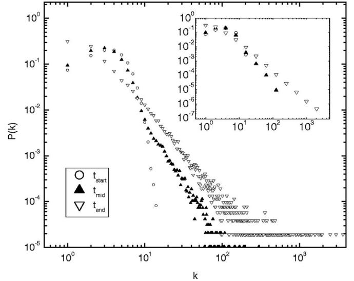
FIG. 2. Node degree distributions of rewired network in three time moments:  $t_{start}=0$ ,  $t_{mid}=2500$ , and  $t_{end}=10\,000$ . Inset: the same data binned logarithmically.
