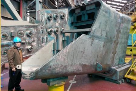
Inner shell assembly of a lower port stub extension for the vacuum vessel.
