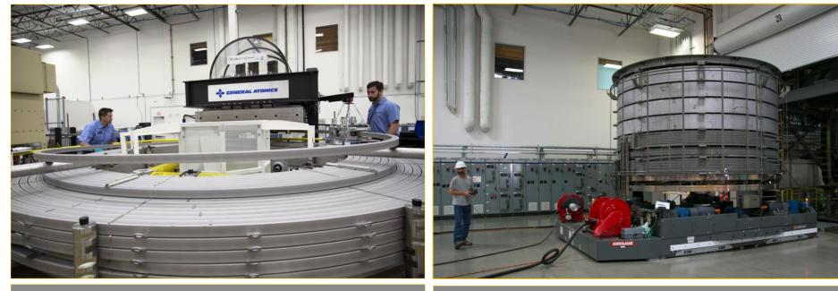
General Atomics is fabricating the 1000-ton Central Solenoid (CS). In April 2016, winding of the first CS module was completed.
