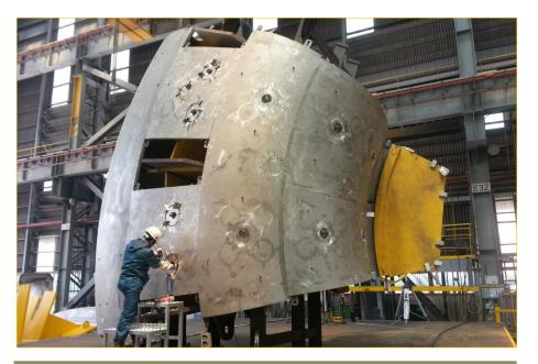
At Hyundai Heavy Industries, where 2 of 9 vacuum vessel sectors are under construction, welding on the upper section of the inner shell for Sector #6.
