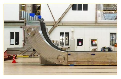
Connection of segments for the first inboard Toroidal Field Coil structure (completed in November 2015), a significant achievement for TF coil procurement.
