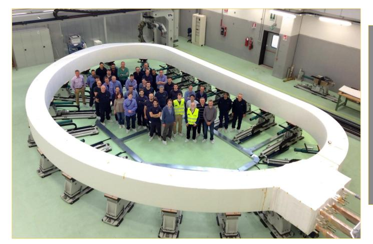
European Domestic Agency contractors have made significant progress in the fabrication of the first toroidal field winding pack—the 110-ton inner core of ITER's D-shaped superconducting Toroidal Field Coils. Following sophisticated, multi-stage winding operations, seven layers of coiled superconducting cable (double pancakes) have now been successfully stacked and electrically insulated.
