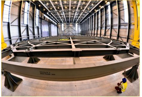
The transportation frame/assembly and welding support for the cryostat has been assembled in the Cryostat Workshop where welding began in August.
