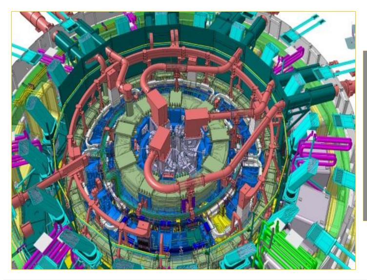
A top view of the cryostat illustrates the high density of sensitive equipment to be installed (e.g., magnet feeders shown in brown, blanket water pipes shown in light blue). A clash free design as well as the access to install and if needed maintain the systems must be ensured by the integration team.
