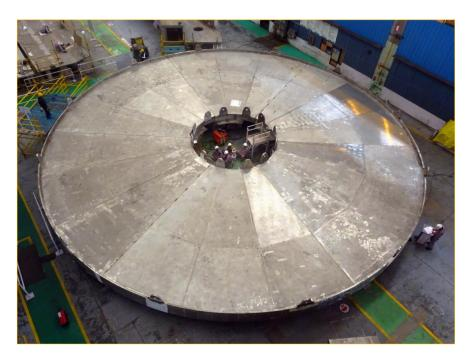
India is responsible for fabrication and assembly of the 30x30 meter ITER cryostat. The base plates were delivered to ITER in December 2015.
