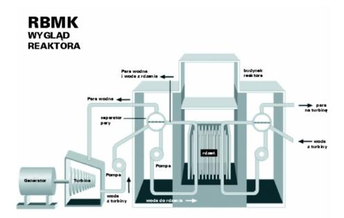
*Fig. 4. Scheme of RBMK reactor.* [2]
