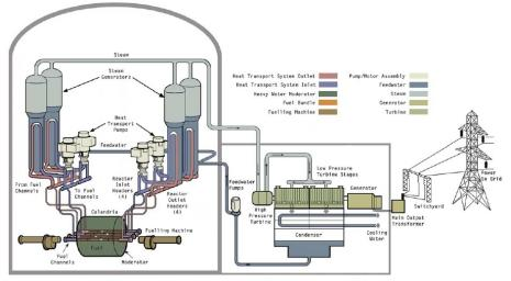
Fig. 3. Scheme of CANDU reactor. [2]
