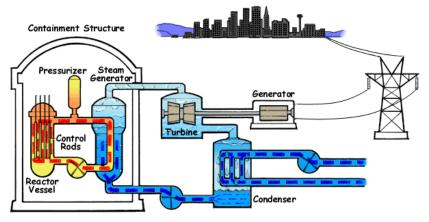
*Fig1. Scheme of PWR reactor.* [1]
