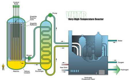
Fig. 5. Scheme of HTR reactor. [1]
