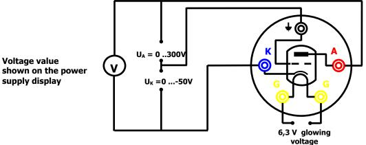
The electric circuit consists of two power supplies:
